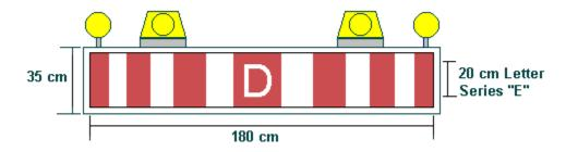
**Box Dimensions** - the box must be 180 centimetres x 35 centimetres x 10 centimetres and constructed of mild steel material with inside and outside surfaces of baked white enamel. The box must shelter all wire connectors, switches, flashers, etc.
