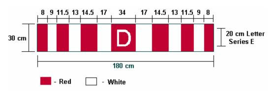
If a lighted sign box is used, it must meet the following specifications:
