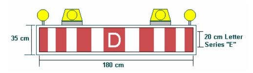
**Box Dimensions** - the box must be 180 centimetres x 35 centimetres x 10 centimetres and constructed of mild steel material with inside and outside surfaces of baked white enamel. The box must shelter all wire connectors, switches, flashers, etc.
