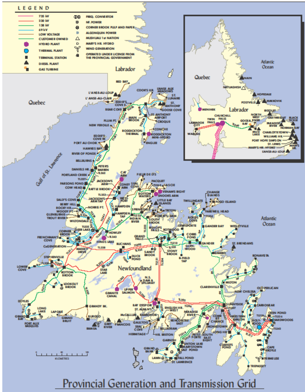
Figure 3: Newfoundland and Labrador Transmission
