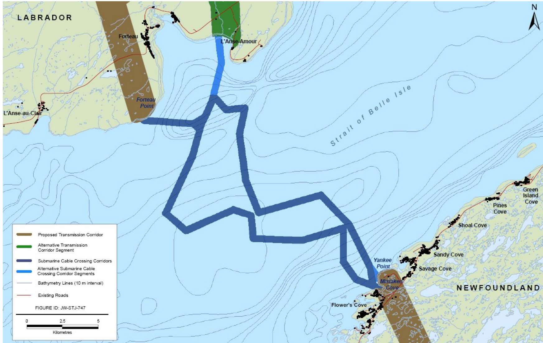
Figure 1-2 Potential landing sites and corridors for Strait of Belle Isle cable crossings (from Nalcor, 2009)
