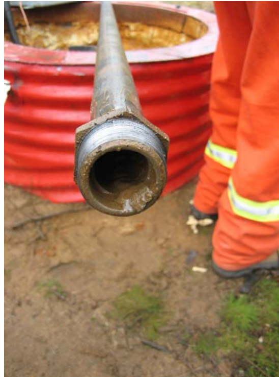
Silt and fines in W4 riser pipe (Site Visit -1)
