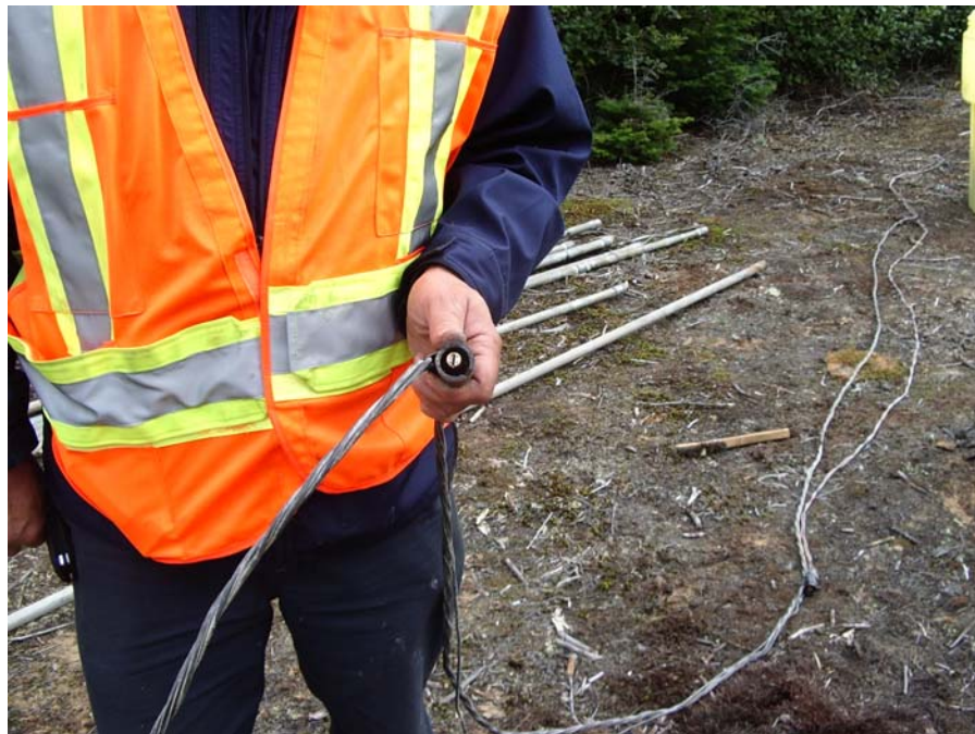
Photograph 6: The four sensors at each well installation were inspected, tested and cleaned. If sensors were in poor condition or malfunctioning, they were replaced.
