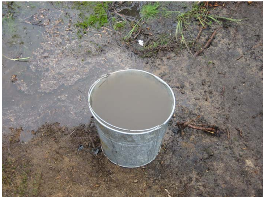
Cloudy water from W4, after pump replacement (2.5 hours of system shutdown) (Site Visit -1)
