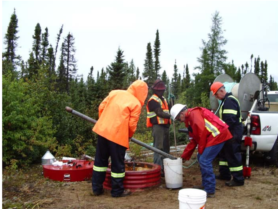
Photograph 9: A sand pump was placed down into the well, water and sediments were suctioned into the sand pump. The sand pump was brought to the surface and the sediments collected in a pail for examination.
