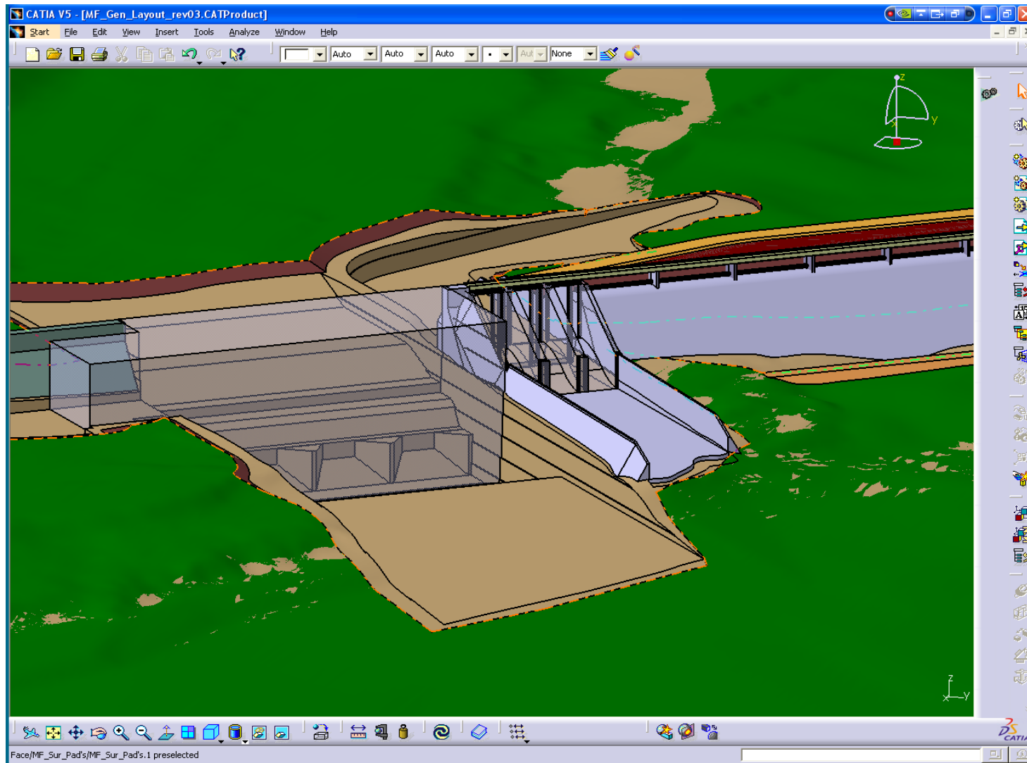
Figure D-1: Base Scheme 1a (3 Surface Vertical Gates 13.75 m Wide with a Rubber Dam) – Sheets 1/4
