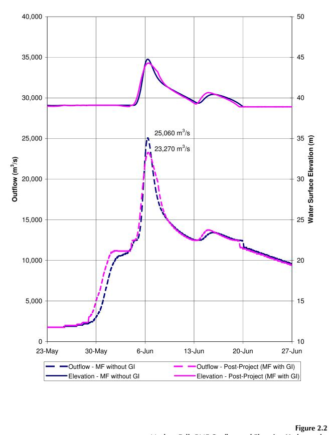
Muskrat Falls PMF Outflow and Elevation Hydrographs MF1330 - Muskrat Falls PMF and Construction Design Flood Study Nalcor Energy - Lower Churchill Project
