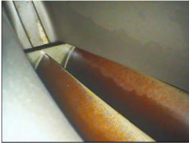
Figure 3: Corrosion on End B Engine
