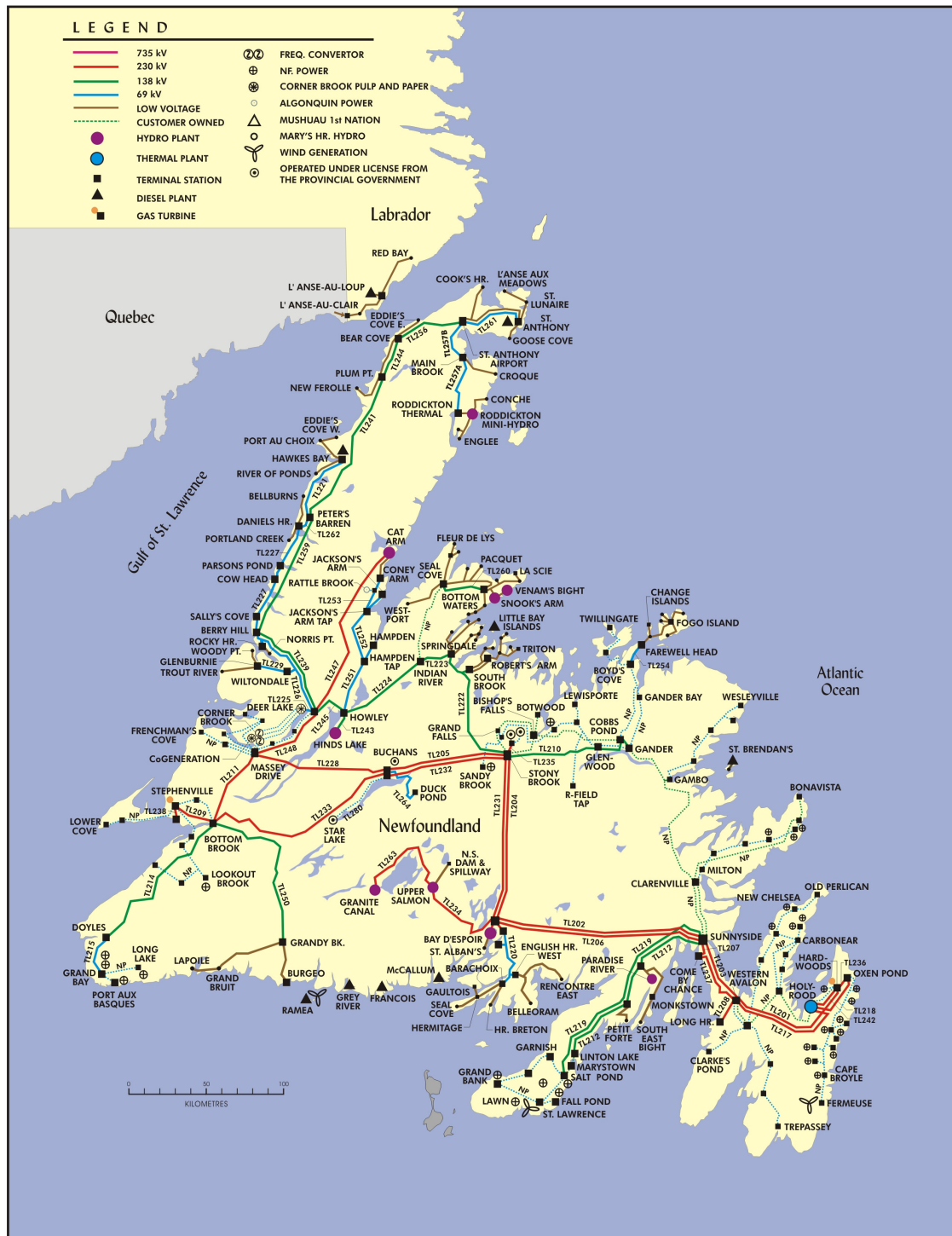
Figure 1 – Island Interconnected Transmission System
