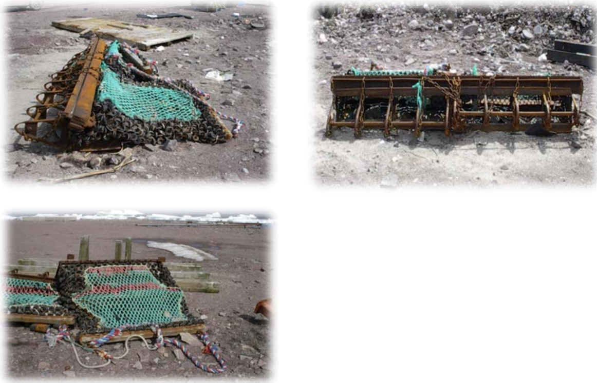
Figure 6. Typical Modified Labrador Scallop Rake used in the Strait of Belle Isle.
