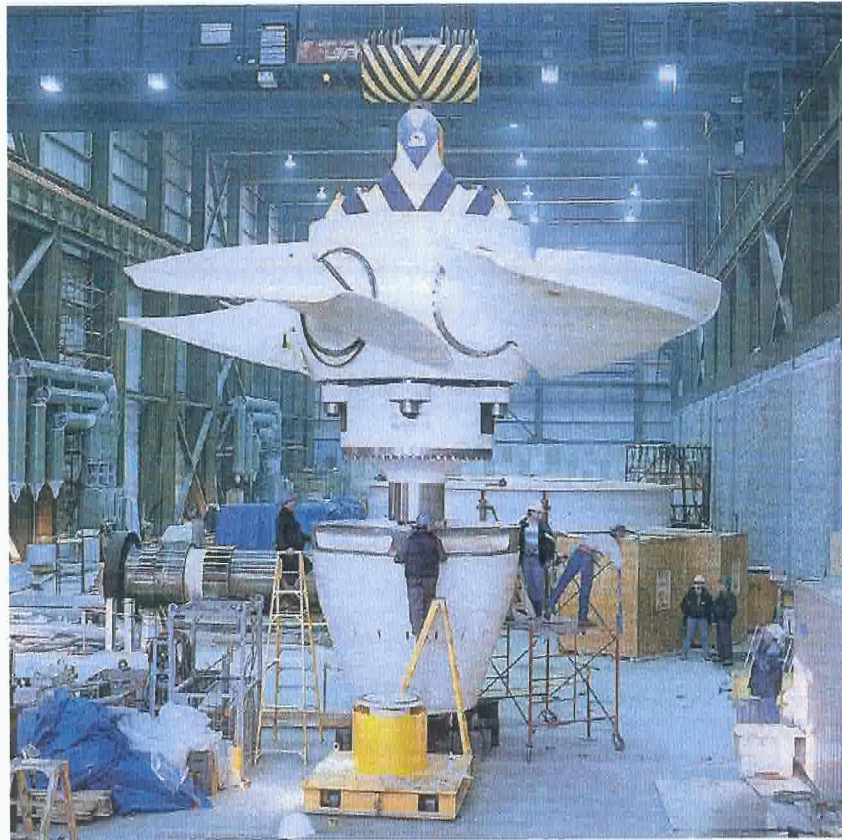
Figure 3-14: Example of a Kaplan Turbine Assembly
