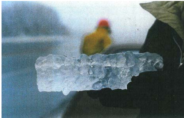
Fig. 2 Glaze ice sample from conductor (1984 storm)
