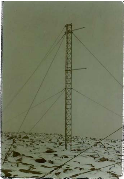
Figure 7. Test tower. Only few towers had two horizontal rods (50 mm) as this tower
