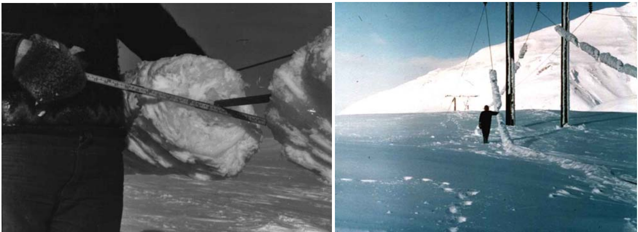
Figure 22. Icing at Hallsteinsvarp 28.02.1978. Ice weight 29.4 kg/m. Density 420 kg/m 3 .
