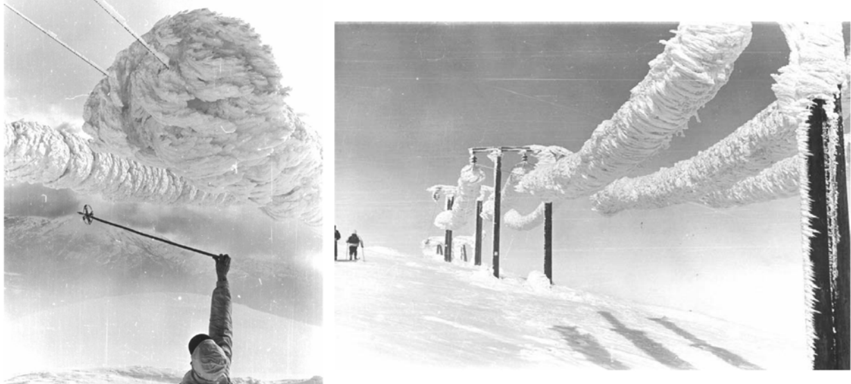
Figure 31. Photo: O. Wist. The most famous photos of in-cloud icing. Ice load 305 kg/m.
