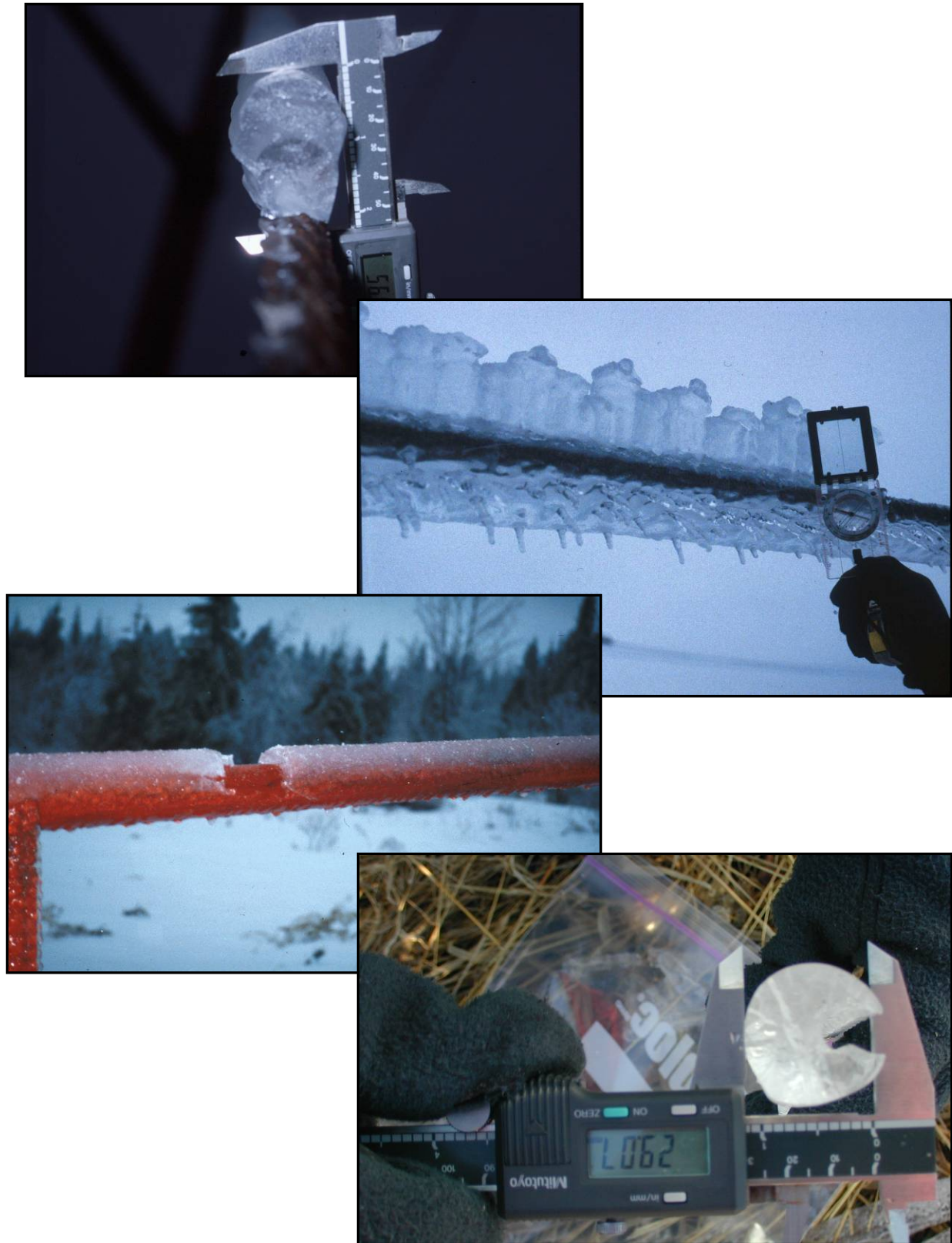
Figure 5. Some of the variety of shapes of ice accreted from freezing rain (photos, CRREL).
